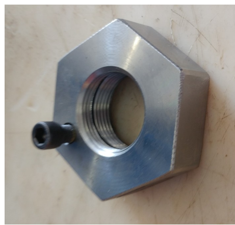
Cap screw will squeeze gap locking the walnut in place
