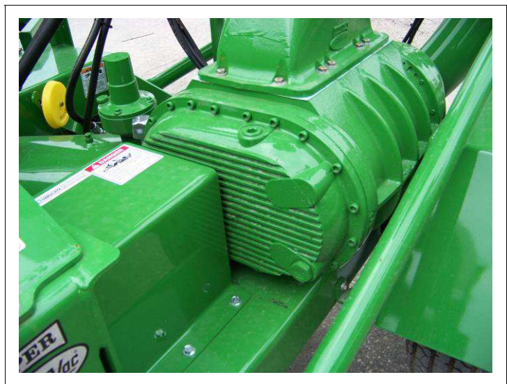
Fig. 5-4 Blower Reservoirs (Front)
