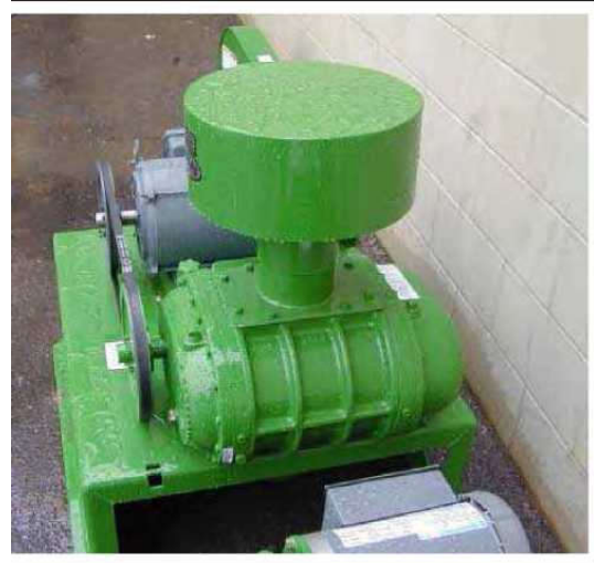
Fig. 5.1 DRIVE BELTS (ALIGNMENT)
