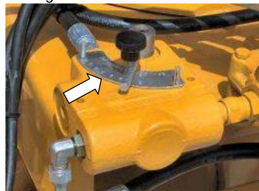
Fig. 4-11 Airlock Flow Divider
