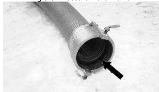
Fig. 5-9 Air Line Seal at Flex Hose
