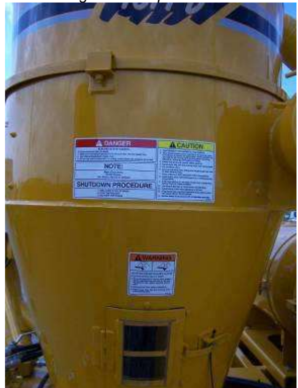
Fig. 4-13 Sight Glass in Receiver Tank
