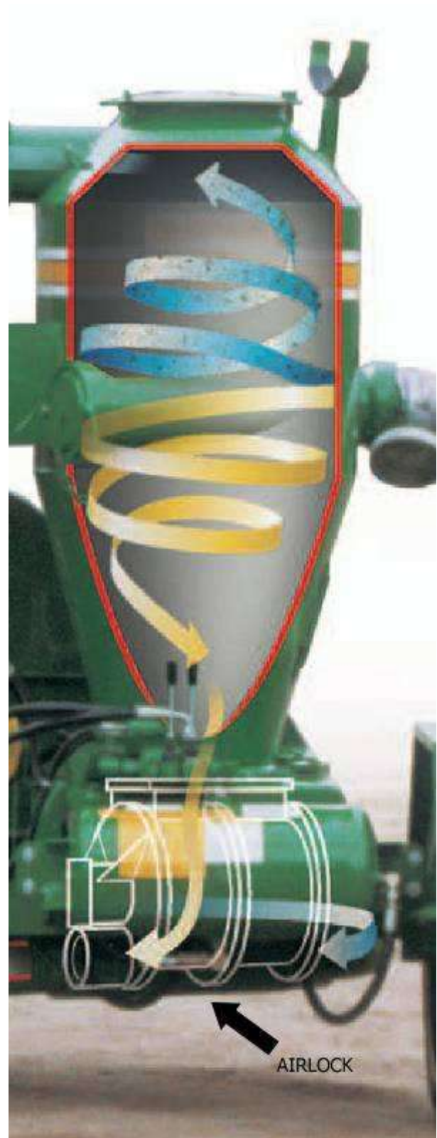
Fig. 5-17 Airlock Typical Location Below Receiver Tank
