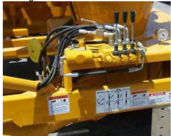
Fig. 4-10 Airlock Flow Divider
