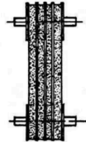
4. For correct installation, both shafts and pulleys are in alignment.
