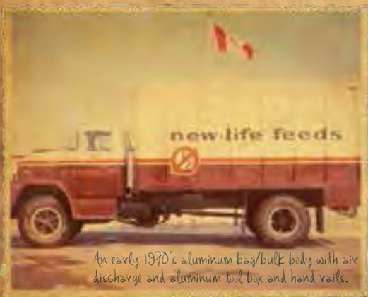
An early 1970's aluminum bag/bulk body with air discharge and aluminum tool box and hand rails.
