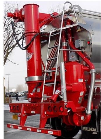
the window, adjust the airlock speed to take the product away faster or open the air slide further to decrease the amount of product being drawn into the suction nozzle.
