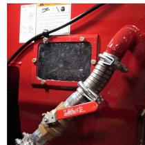
16. Insert the suction nozzle into the product with the inlet below the surface of the product, but ensuring that the suction nozzle slide is not covered.
