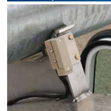
Boom out of saddle light
