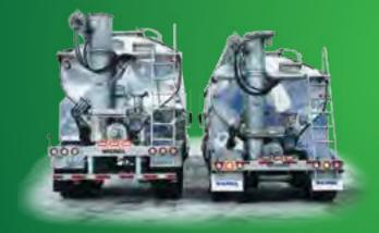
Tanks are now lower to the ground and more stable to reduce rollovers. By reducing the height or lowering the centre of gravity, the unit is more stable.
