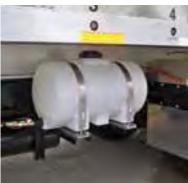
Feed trailers are optioned with cab actuated disinfectant spray systems that douse tires to inhibit the spread of disease from one farm to another.
