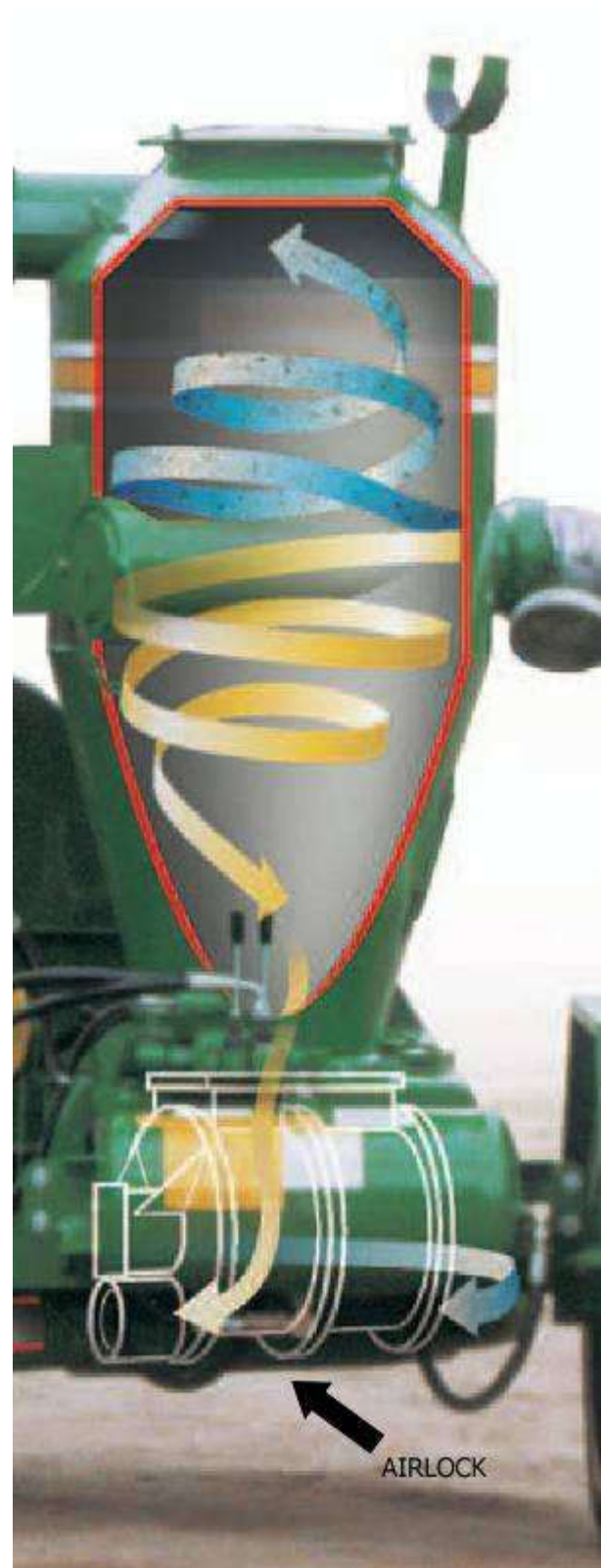
Fig. 5-17 Airlock Typical Location Below Receiver Tank
