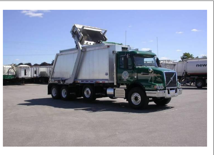
Fig. 4-15 Dumping Bucket Into Box
