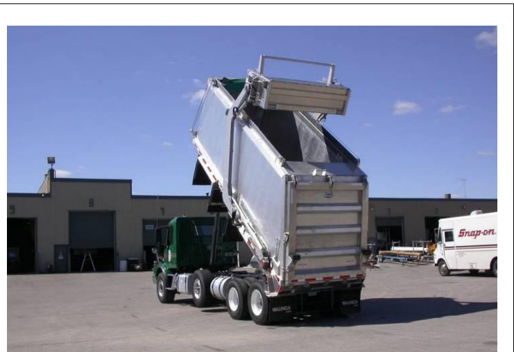
Fig. 4-16 Box Up With Bucket Raised
