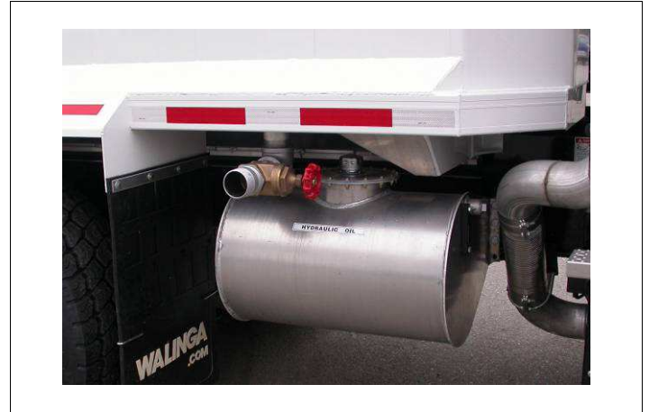
Fig. 7-6 Hydraulic Tank (Typical)
