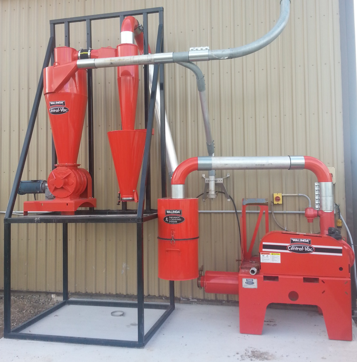
Typical Central Vac Set Up
