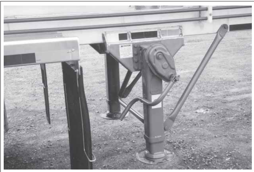
Fig. 6-7 LANDING GEAR MOUNTING BOLTS
