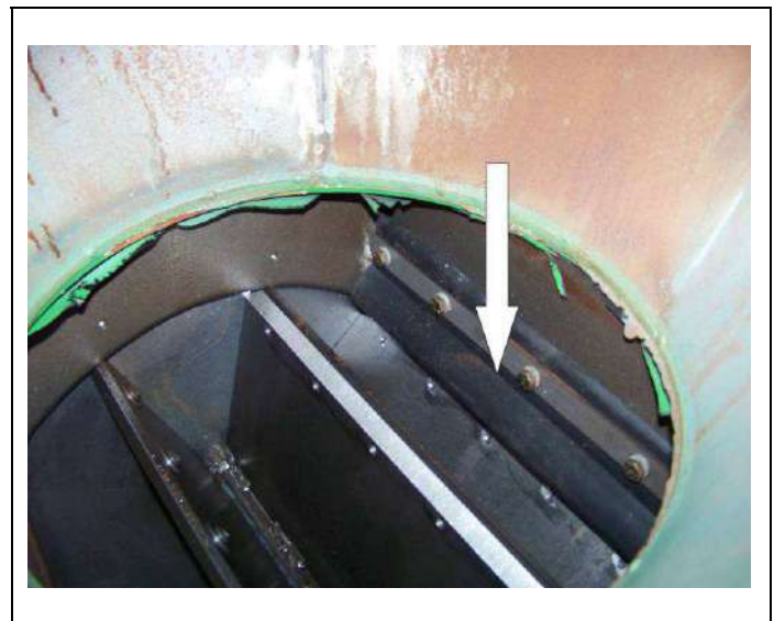
Fig. 5-28 Check Wiper Blade Through The Access Door
