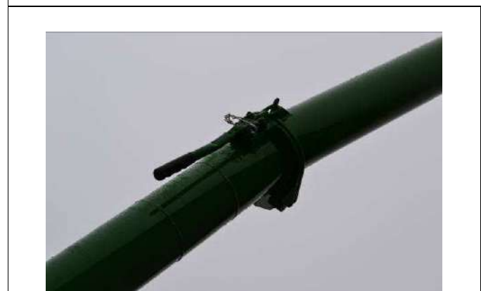
Fig. 4-12 Coupling Upper Boom & Mid Boom
