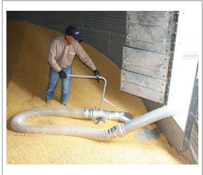
Fig. 4-20 Using The Clean-Up Nozzle In the Bin.
