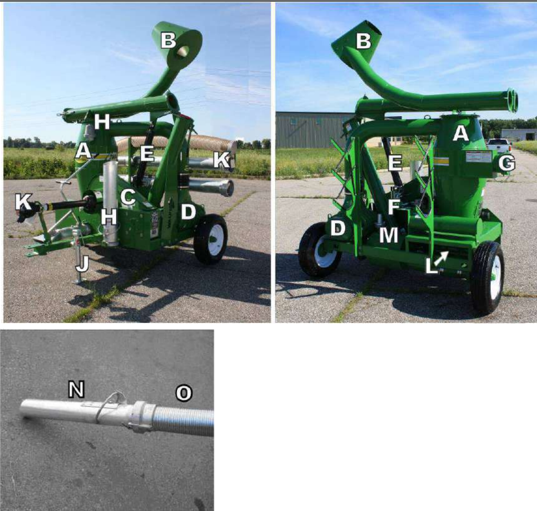
Fig. 4-1 Components - 7614F In Transport Mode.
