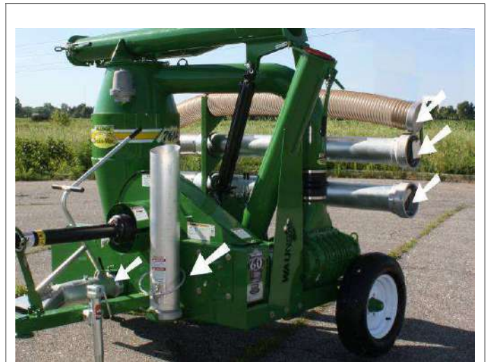
Fig. 4-21 Nozzle and Hose Storage
