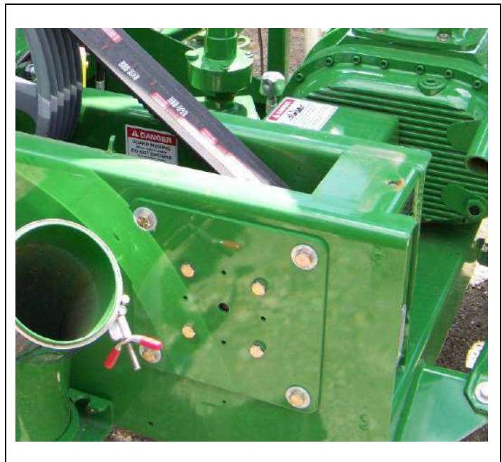
Fig. 5-20 Adjusting Anchor Bolts At Bearing Housing Assembly.
