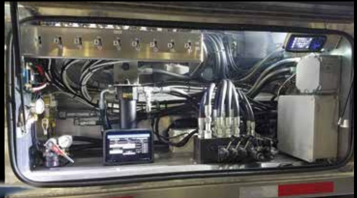
Specially designed electronic hydraulic controls maximize flow/pressure for optimum performance. All utility boxes are manufactured from aluminum, are positioned for easy access and include wiring diagram labels.
